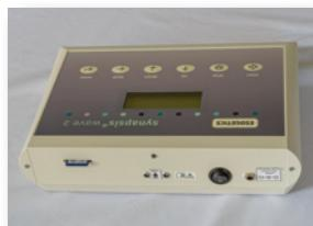
Remove the SD card from the instrument. A slight pressure will activate the spring-loaded mechanism to eject the card from the device (illistr. 11)
